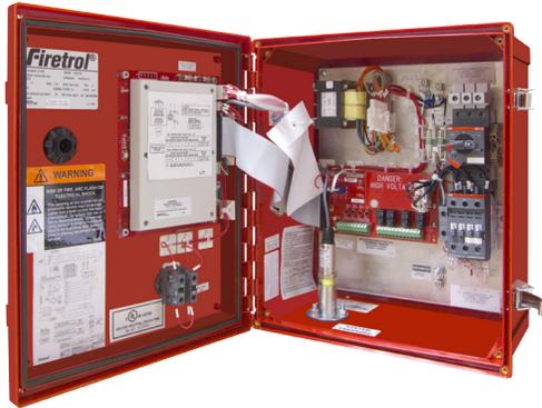
**Description**—Firetrol® FTA550F XG Jockey Pump Controllers are intended for use with fire pump systems. They are used for pressure maintenance in fire pump installations to prevent unnecessary operation of the main fire pump.
