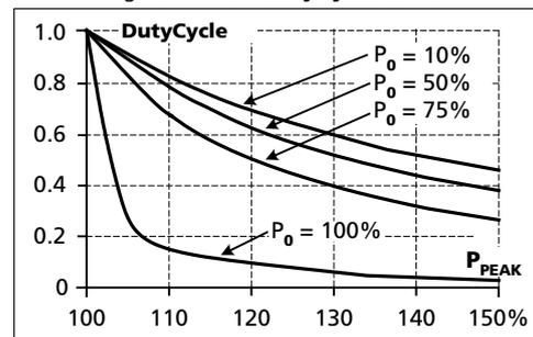
$$\text{DutyCycle} = \frac{T_{\text{peak}}}{T_{\text{peak}} + T_0}$$
