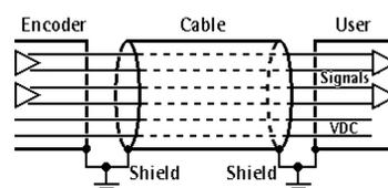
Wires not used must be cut at different lengths and insulated singularly
