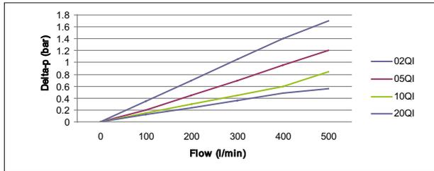
**EPF Size 4 Length 1 Filter Elements with reverse flow valve**
