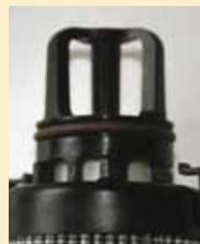
A new design of the filter element allows integration of the bypass valve and element core as re-usable parts in the filter bowl. This results in cost reduction when integrating the high pressure filter in manifold type solutions. But it also reduces the waste when changing the filter element by over 50% as the element core is an integral part of the filter bowl.
