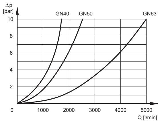
**4.2 - Flow control function with damping nose LC\*-QD**
