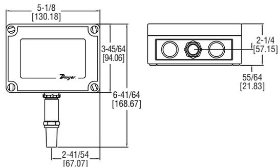
The Series RHP Humidity and Temperature Transmitter offers flexibility, high accuracy, long term stability, and reliable operation. Utilizing the duct and outside air mounting configurations, the Series RHP monitors and controls humidity or both humidity and temperature in a building energy management systems, commercial and residential HVAC applications, clean rooms, museums, and climate chambers.
