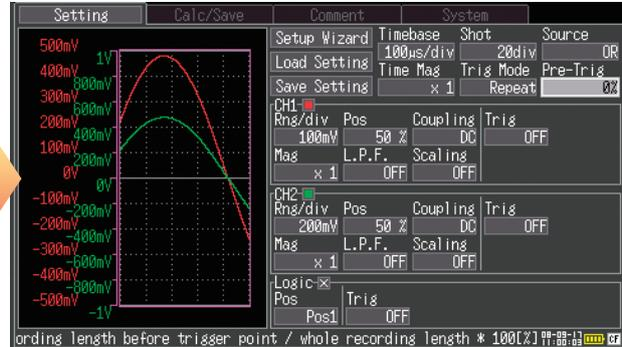
The help text crawls along the bottom of the screen, describing the function of the setting at the blinking cursor. The enhanced "Waveform Monitor" window with level meter display facilitates changes to settings by simultaneously displaying real-time input waveforms.
