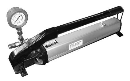
The powerful high pressure oil pump is used for professional operation of hydraulic clamping elements equipped with oil nipple.
