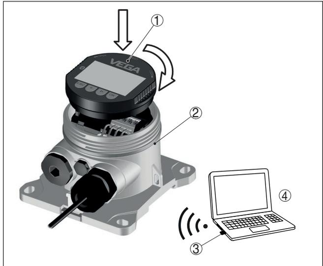
Fig. 26: Connection of the PC via Bluetooth USB adapter
