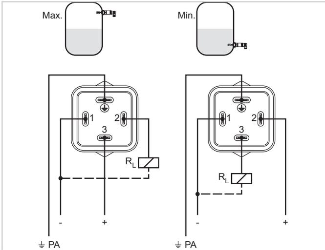
VEGASWING 51 with valve block according to ISO 4400
