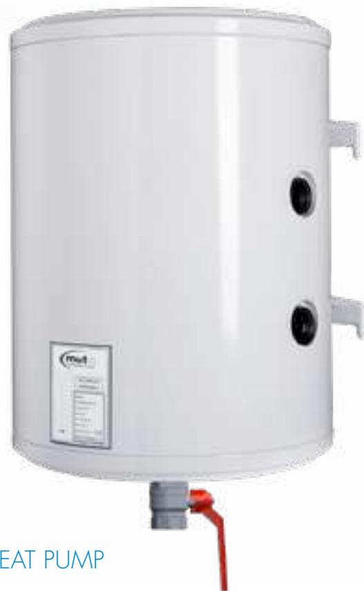
Mut inertial storage units are devices designed to connect heat pumps and other heat generators to multiple booster sets. They make it possible to optimise the performance of heat pumps, limiting the switching on and off cycles that affect their life expectancy as well as their efficiency, and at the same time speed up defrosting cycles during the winter period.
