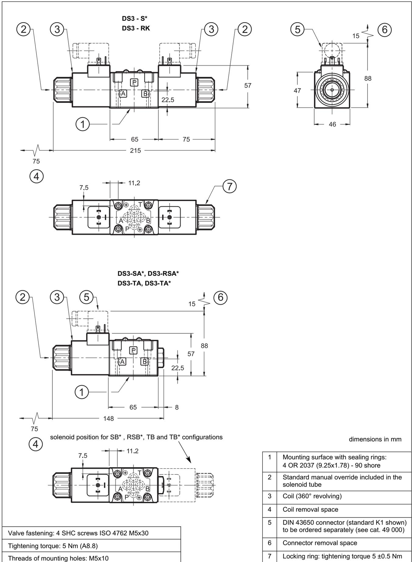
9 - OVERALL AND MOUNTING DIMENSIONS FOR AC SOLENOIDS VALVES
