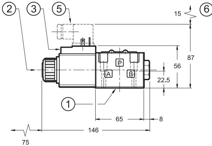
4 solenoid position for SB\*, RSB\*, TB and TB\* configurations
