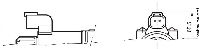
connection for DEUTSCH DT06-2S male connector - coil with diode
