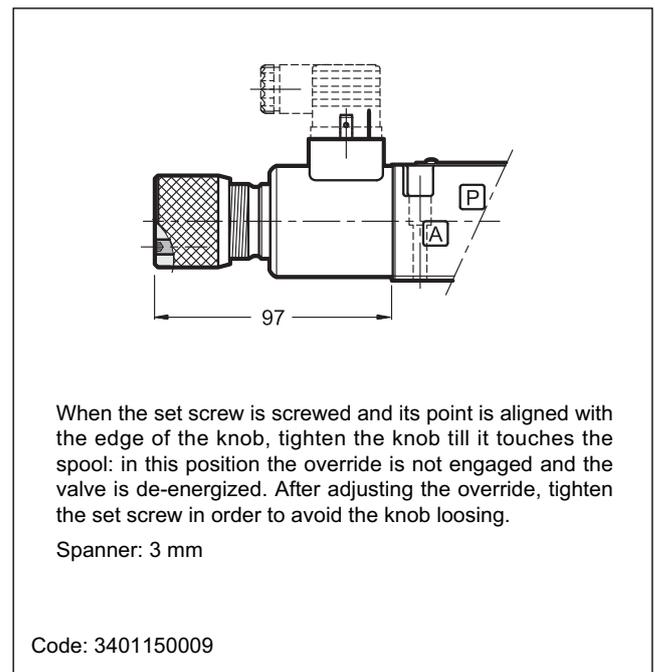
13.5 - CPK-DS3/10 Push manual override with mechanical retention (only for DC solenoid valve)
