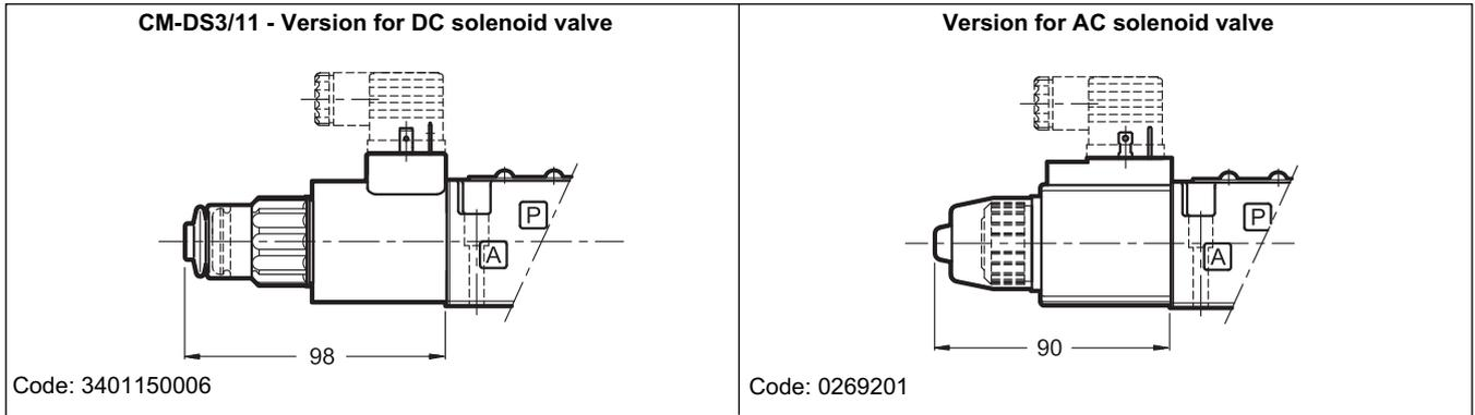
13.2 - CH-DS3/11 Lever manual override (only for DC solenoid valve)
