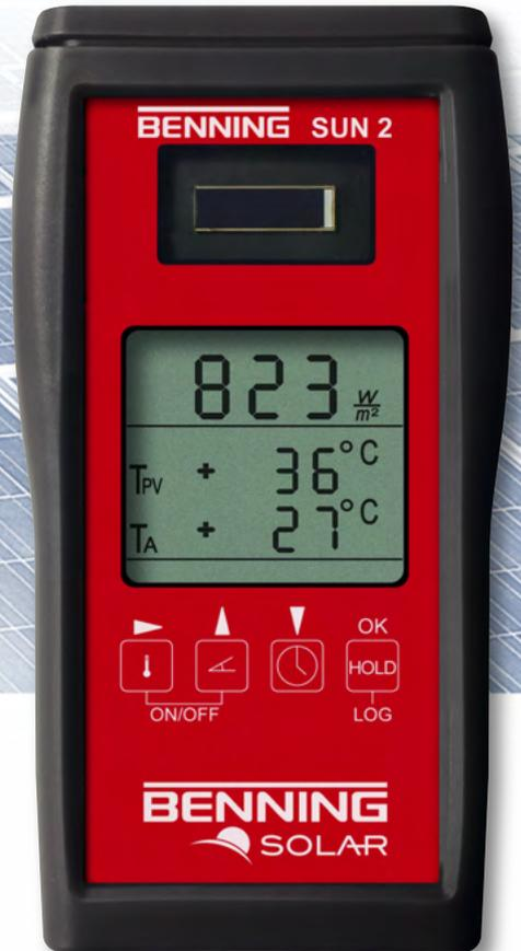
Insolation, PV module/ambient temperature
