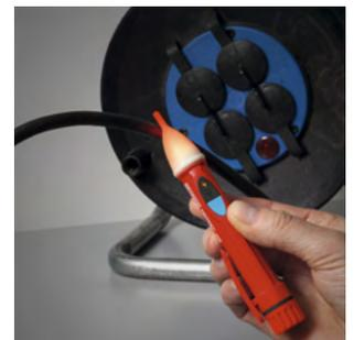
Testing of cable breaks
