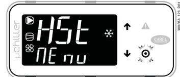
Category Hst (Alarm log): access the alarm log. Each event is described with the date (in the format DD MM) and time (in the format hh:mm) alternating.
