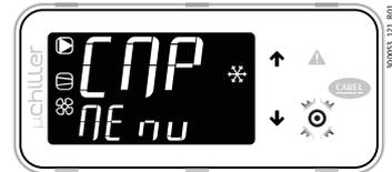
Category CMP (compressors): identified by code Cxxx, these parameters all relate to control and management of the compressors and refrigerant circuits.
