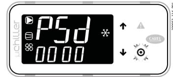
3. Press PRG: the first digit of the password flashes; set the value, press PRG. The second digit now flashes; enter the other digits to complete the password.
