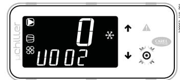
6. Press PRG: the value flashes; press UP/DOWN to change the value; PRG to confirm.
