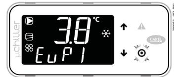
Press DOWN: EuP1 indicates the evaporation temperature in circuit 1 (3.8°C).
