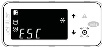
To return to the standard display, press PRG (corresponding to ESC).
