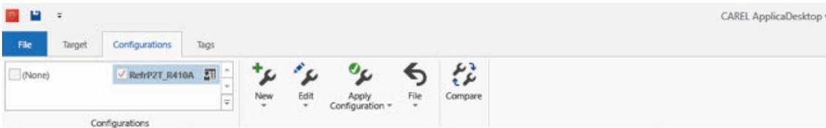
Finally, to save the newly-created configuration for future use, from the "Configurations" label select "File -> Export" and assign a name to the configuration being saved.
