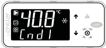
Press DOWN: Cnd1 indicates the condensing temperature in circuit 1 (40.8°C).
