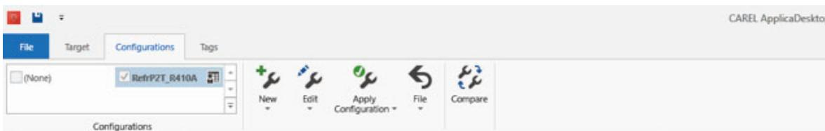
3. Applica Desktop will display a message when the parameters have been set, and if necessary indicating any values that have been applied that do not belong to the current user profile (some parameters may not be visible to the user).
