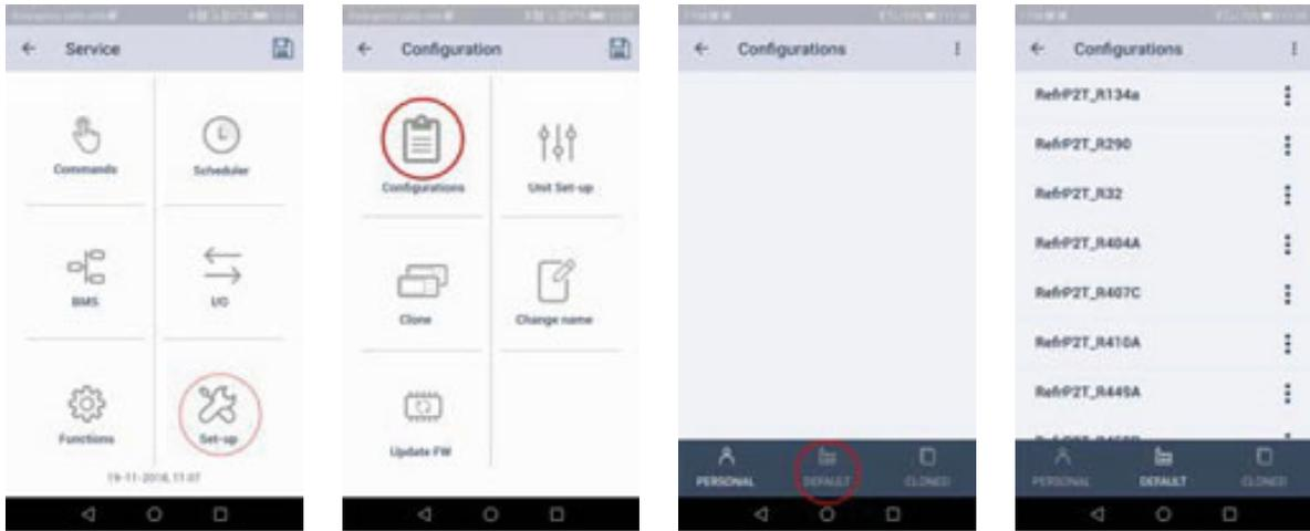
4. apply the selected configuration via NFC or Bluetooth. The refrigerant has now been correctly configured.
