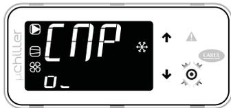
Press DOWN: CMP indicates that compressor 1 is on (o) and compressor 2 is off (□).
