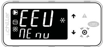
Category EEV (ExV valve): identified by code Exxx, these parameters all relate to control and management of the electronic expansion valve (s).
