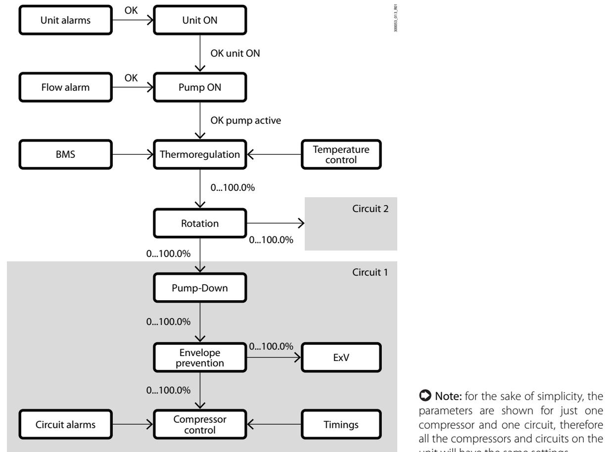
**Note:** for the sake of simplicity, the parameters are shown for just one compressor and one circuit, therefore all the compressors and circuits on the unit will have the same settings.
