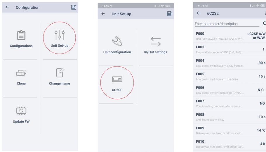
2. apply the parameters configured via NFC / Bluetooth to the controller.
