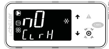
9. Press DOWN: the function to delete the alarm log (ClrH) is shown - Service level only.
