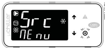
Pressing the Alarm button for more than 3 s resets the alarms: noAL indicates that there are no more active alarms. Press PRG to exit the alarm list.
