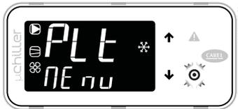
When an alarm is active, the buzzer sounds and the Alarm button lights up
