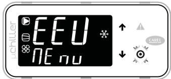
Pressing Alarm mutes the buzzer and displays the alarm code; pressing UP/DOWN scrolls the list of any other alarms.
