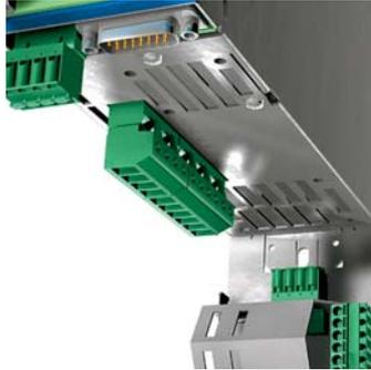
The separate connections for motor, DC link and braking resistor are located on the bottom of the housing. The PTC thermistor and braking relay are also attached here by simple plug-in mounting.
