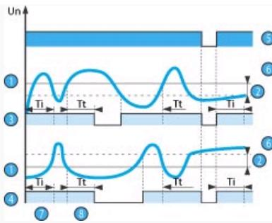
In overcurrent mode, if the controlled current exceeds the preset threshold for longer than the time set on the front face (0.1 to 3 s), the output relay opens and LED R is extinguished. During the time delay, this LED flashes.
