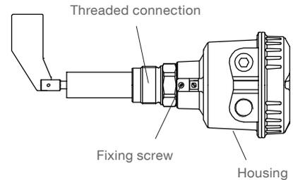
**Direction of the cable glands** When the unit is mounted from the side, ensure, that the cable glands face downwards and are closed to avoid water penetration into the housing.
