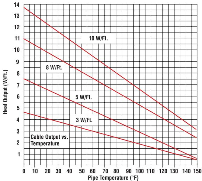
**Note 1** — Thermal output is determined per IEEE 515-1997 Standard for testing, design, installation, and maintenance of electrical resistance heat tracing section 4.1.11 Method C.
