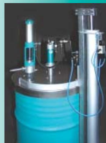
Complete installations with pneumatic lift, pumps and agitators are available
