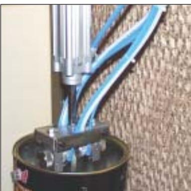
Spray guns mounted on lifting device to carry out spot repair
