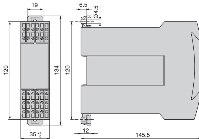
Fig. 7. SINEAX VC 603 in housing **S35**, with the screw hole brackets pulled out for wall mounting.
