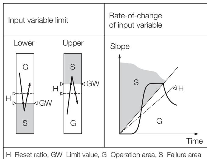
Fig. 5. Switching function according to limit monitored.
