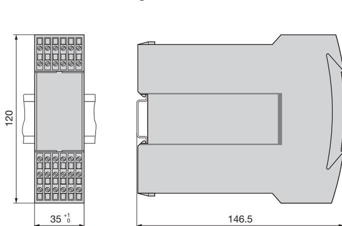
Fig. 6. SINEAX VC 603 in housing **S35** clipped onto a top-hat rail (35 × 15 mm or 35 × 7.5 mm, acc. to EN 50 022).
