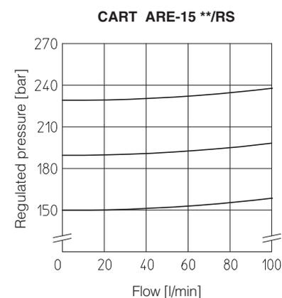
**8 REGULATED PRESSURE VERSUS FLOW DIAGRAMS** (based on mineral oil ISO VG 46 at 50°C)
