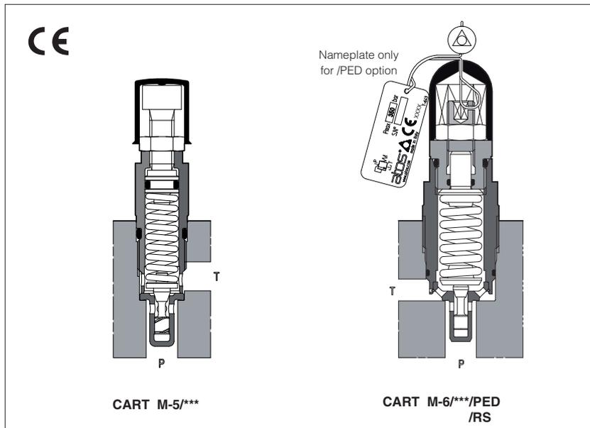
**CART** are direct operated pressure relief valves for screw-in mounting. They are used to limit the max pressure in the hydraulic systems or to protect part of the circuit from overpressure. They are available in six sizes for different flow and pressure range. The cartridge execution is specifically designed to reduce the dimension of blocks and manifolds, without penalizing the functional characteristics.
