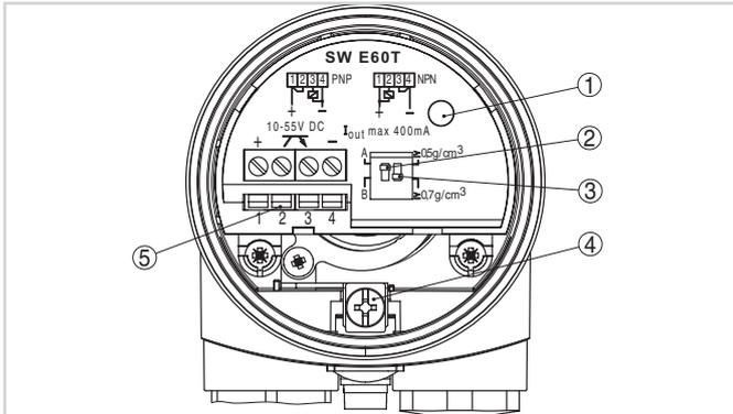
Electronics and terminal compartment, single chamber housing
